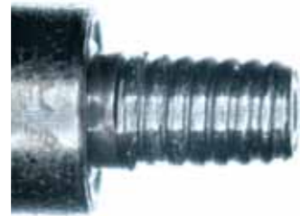
DAMAGED → Generic ultrasonic instruments overload the sonotrode and severely shorten its life span
